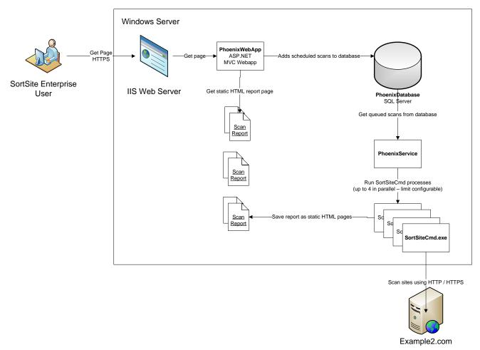
The basic architecture of Enterprise Suite is shown above. The main components are:
